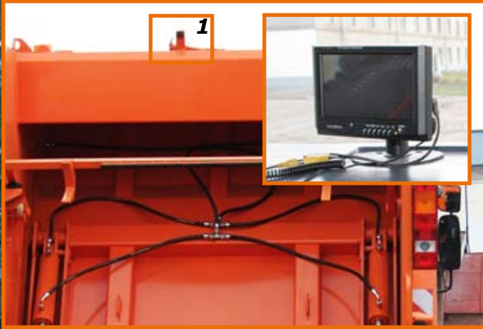
Video camera (1) connected to on-board computer (2) allows controlling refuse truck operation
