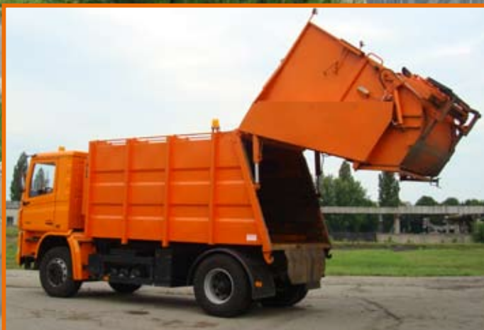
Waste unloading using ejector plate with raised loading hopper
