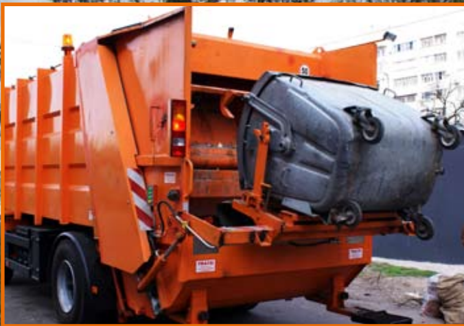
Waste loading from containers using loading device with lifting capacity of 700 kg
